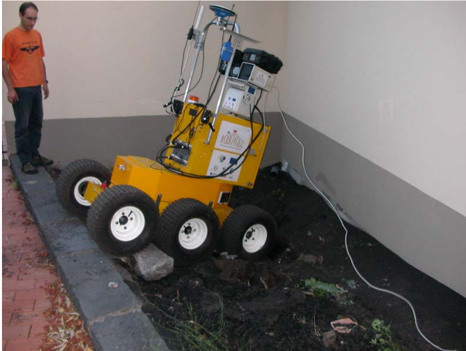
Fig. 28 Traction control test at INGV laboratory in Nicolosi
