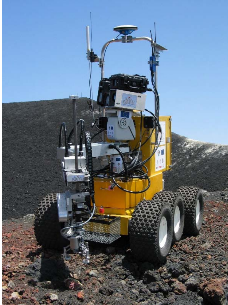
Fig. 21 Manipulator and pan-tilt turret
