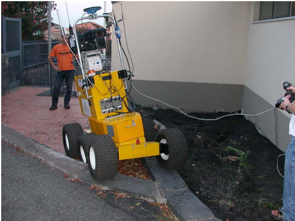
Fig. 29 Climbing capability test at INGV laboratory in Nicolosi
