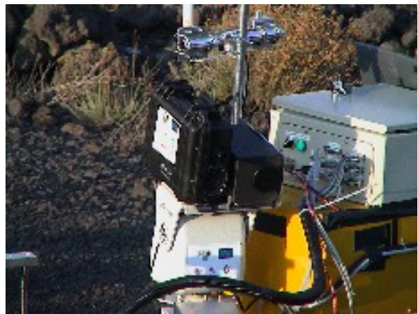
Fig. 14 Gripper and pan-tilt with Digital videocamera and IR camera
