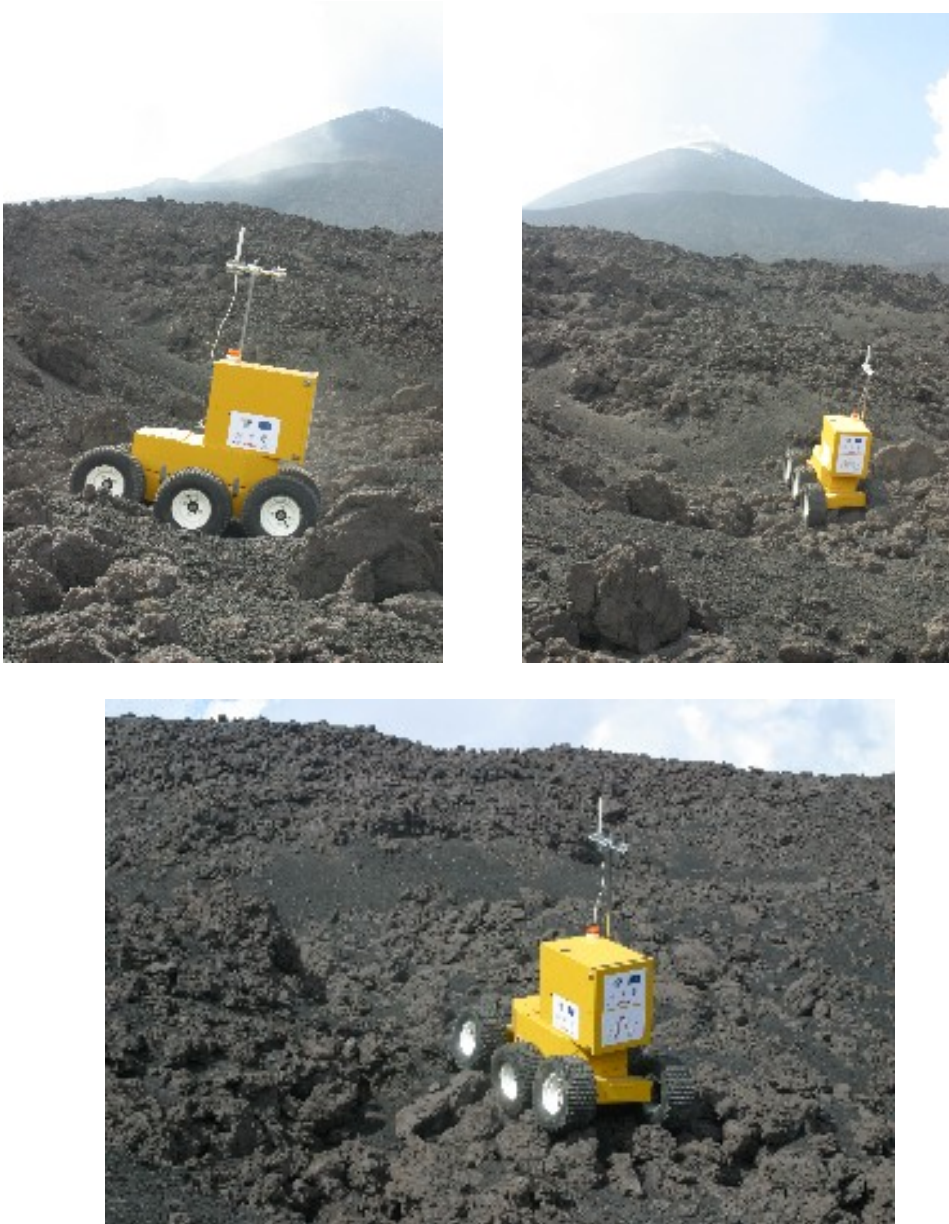
Fig. 17 Trials of the vehicle on hard lava surface (3000m altitude) at Piano delle concazze ETNA.
