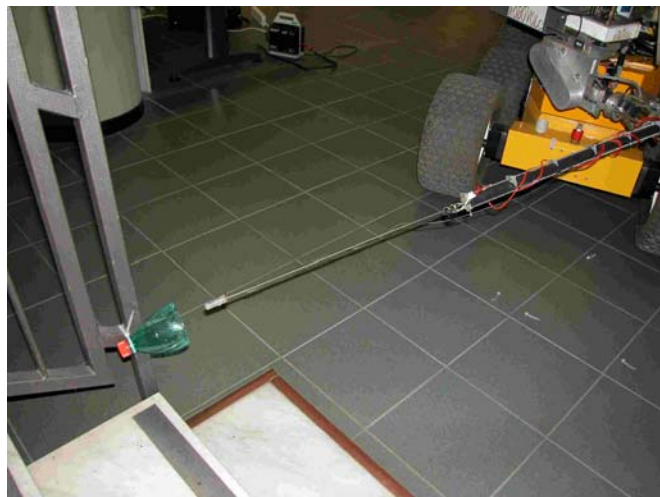
Fig. 42. Test of gas sampling procedure in laboratory.
